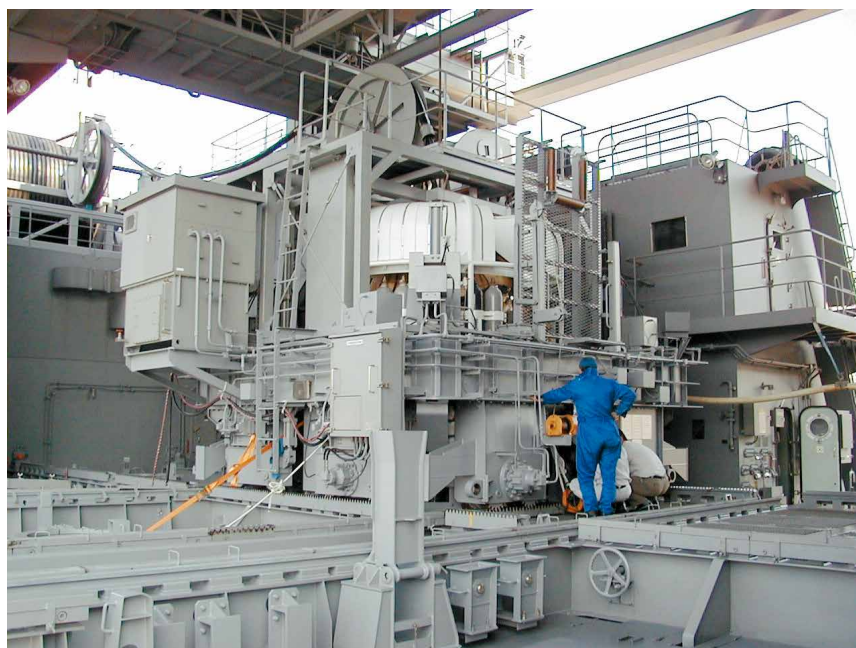
深海潜水装置 (PTC) 用移動・揚降装置 潜水艦救難艦「ちはや」に搭載 Deep sea diving craft (PTC) moving/lifting system installed on "Chihaya", submarine crash boat
