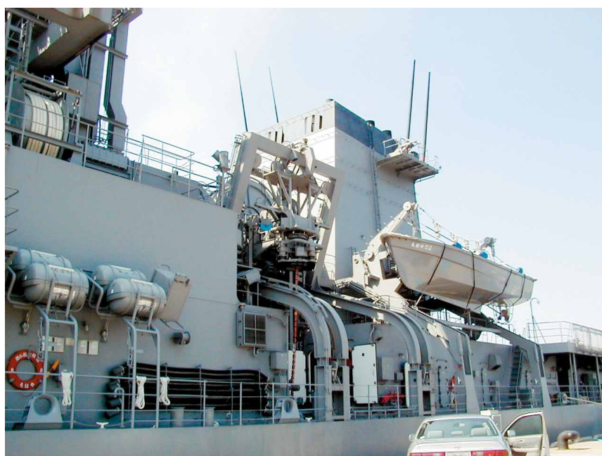
深海潜水装置 (ROV) 用舷側揚収装置 潜水艦救難艦「ちはや」に搭載 Ship-side lifting/accommodation system for deep sea diving craft (ROV) installed on "Chihaya", submarine crash boat
